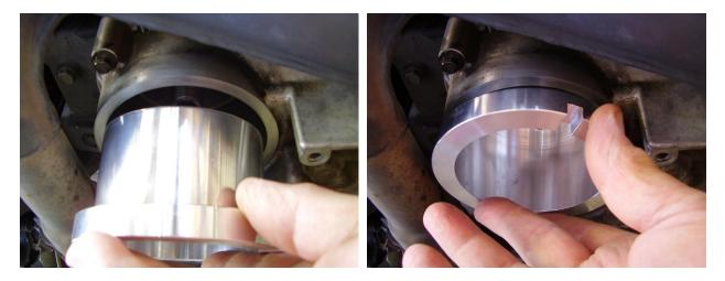
**7.13** Thread the **Housing** *up to but not quite touching* the engine oil cavity flange. The adhesive/sealant being used is of an anaerobic type and will not cure until it is in the absence of air. Bringing the flange into contact with the engine oil cavity flange may start the curing process and this should start only when you are in position to tighten and torque the **Housing** into place. Be sure the O-Ring stays properly inserted in the groove while tightening.
